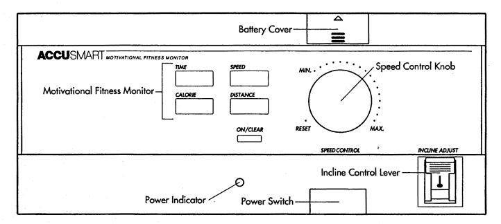
The CROSS WALK features the innovative ACCUSMART console, designed to help you get the most from your workouts. The ACCUSMART console offers electronic speed control, finger-touch incline control and a motivational fitness monitor with four independent displays. Please read the instructions below before operating the console. Note: If there is a sheet of clear plastic on the face of the console, remove it before operating the console.
